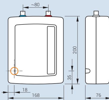
Raccordement d'eau: M 3/8"
